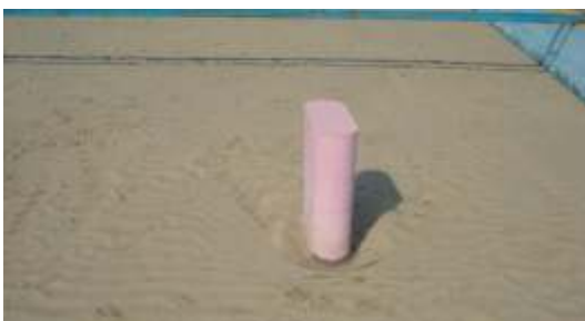
View of scour around pier at 90° flow for f = 8.222
