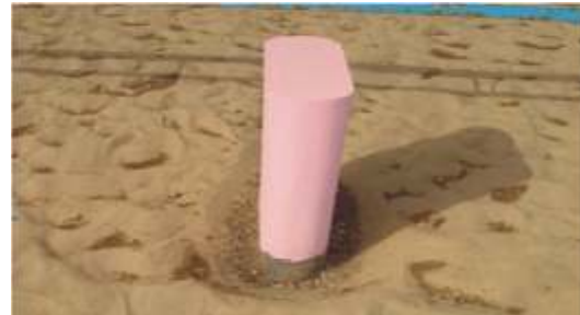
View of scour around pier at 90° flow for f = 9.297
